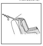
If the position you are using does not have a head restraint and you are using a single tether, route the tether over the seatback.
